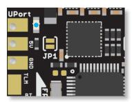
**Receiver input:** Connect your 3-wire (S-Bus, Spektrum, PPM ...) receiver signal port to the "UPort". The receiver's telemetry wire goes to the "RC TLM" on top of the board.
