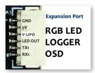
**Expansion Port:** Can be used for serial in/output (RX1 / TX1), e.g. logger or OSD, WiFi connection and LED support. The 5V output can handle 1A max.
