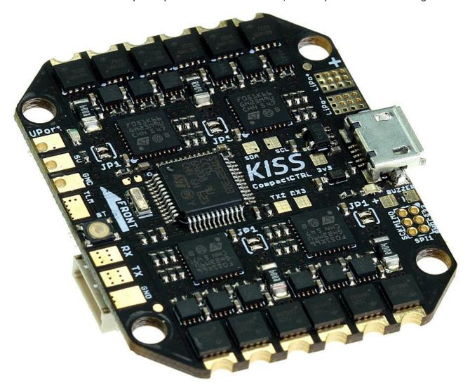
The KISS CC should be ideally driven up to 4s and up to 4 inch props. 5 inch props are possible but you need to choose motors carefully. The CC will actively limit the output to 21A.
